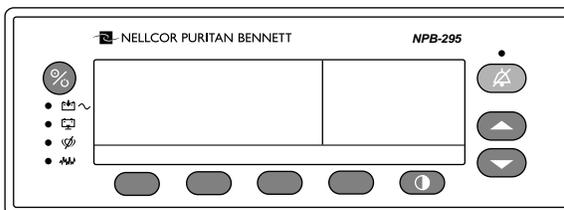
**Figure 4-1: Service Function Softkeys**
