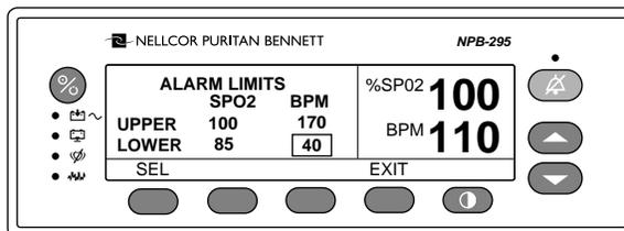
**Figure 3-6: Adjusting Low Pulse Rate Alarm**
