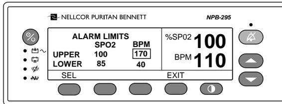
**Figure 3-5: Adjusting High Pulse Rate Alarm**
