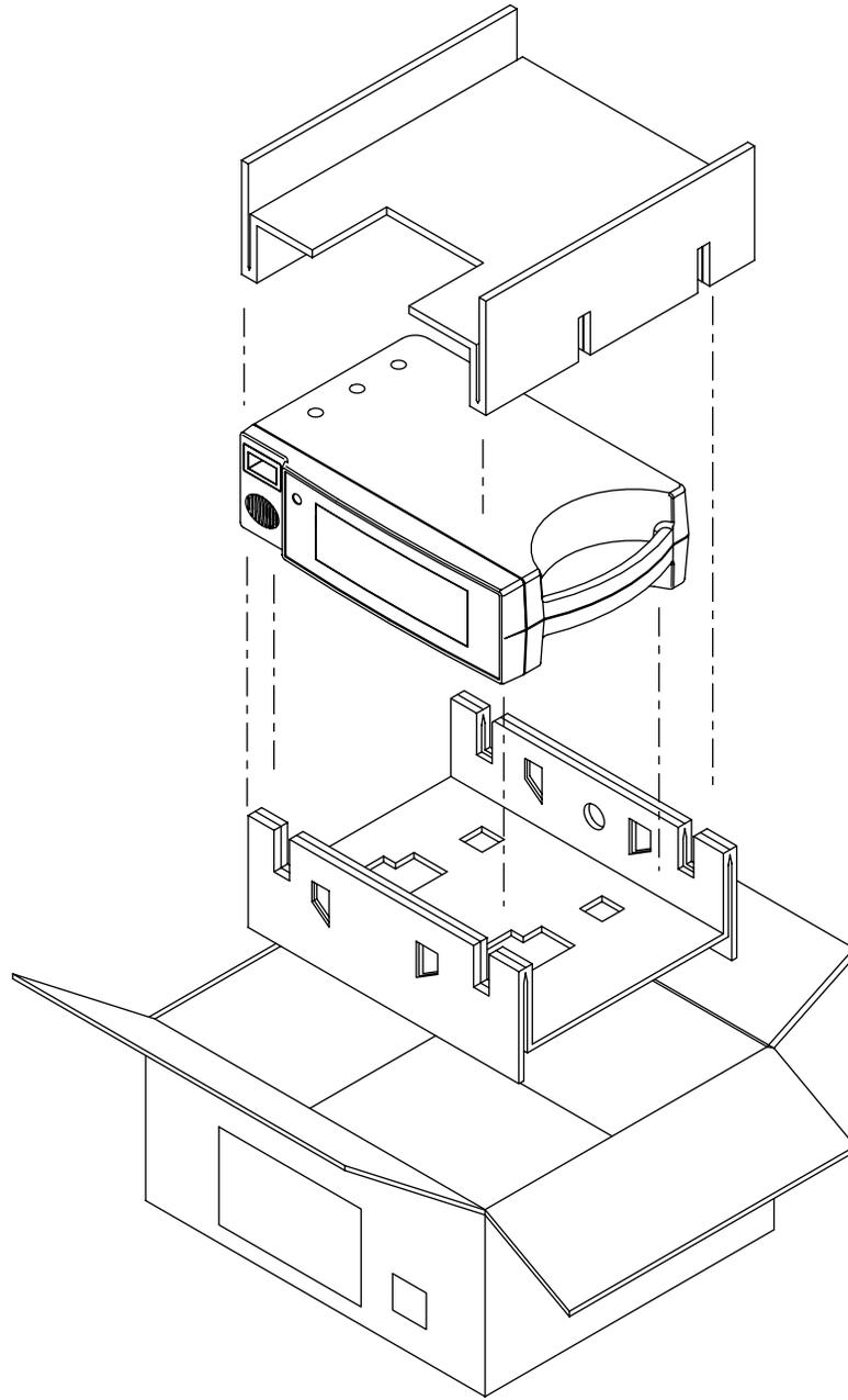
**Figure 8-1: Repacking the NPB-295**
