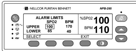
**Figure 3-3: Adjusting %SpO<sub>2</sub> Upper Alarm Limit**
