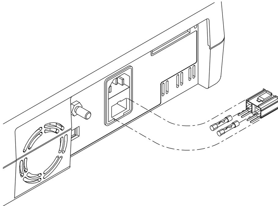
**Figure 6-1: Fuse Removal**
