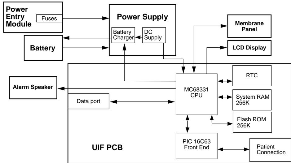
**Figure 11-2: NPB-295 Functional Block Diagram**
