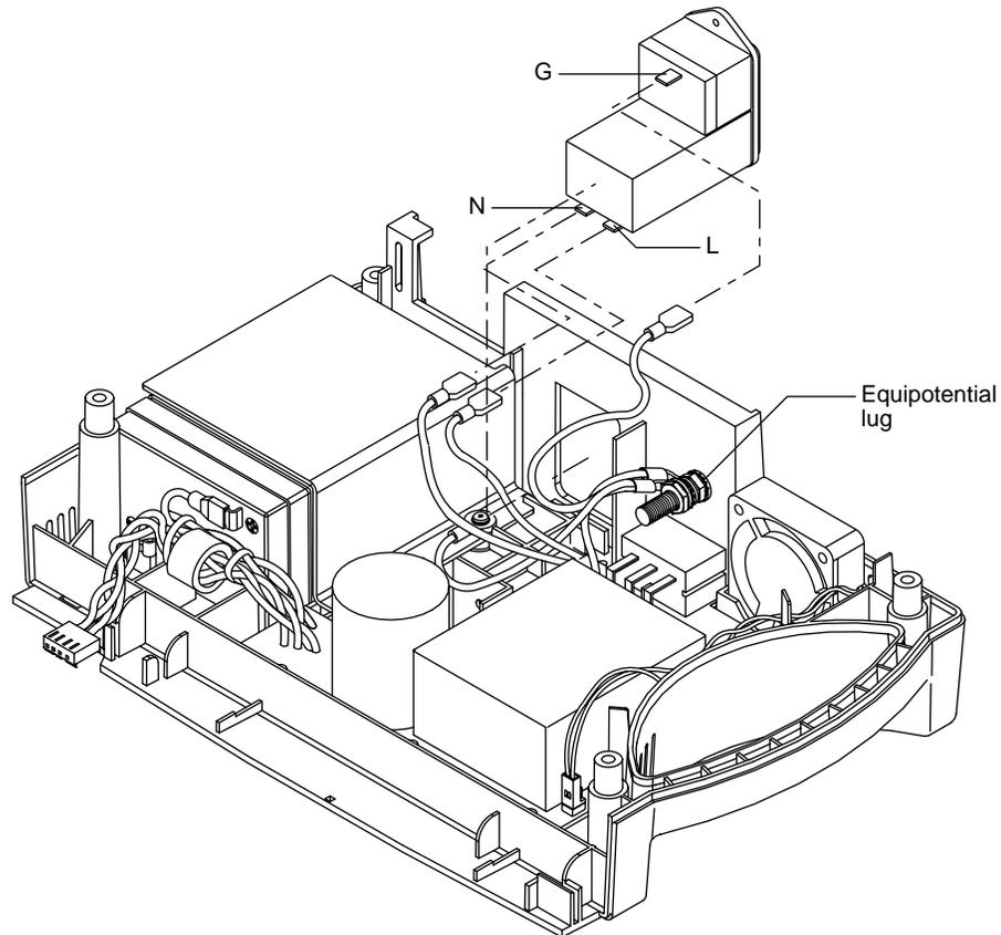
Figure 6-5: Power Entry Module
