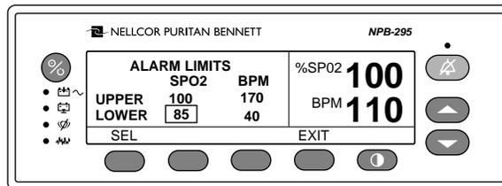
**Figure 3-4: Adjusting % SpO<sub>2</sub> Lower Alarm Limit**
